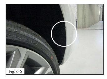
(f) Ensure that the wheel well lining is inside the edge of the bumper fascia (Fig. 6-6).
