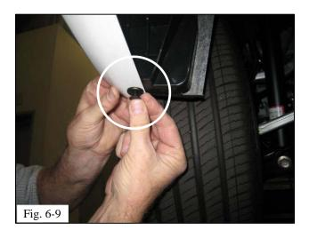
(g) Insert the four lower center bumper fascia push pins (Fig. 6-7).
