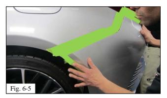
(e) Align the bumper fascia at the wheel wells and push until the small tabs engage (Fig. 6-5).
