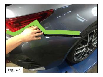
(d) Detach the bumper fascia from the vehicle by pulling from the wheel well on each side.(Fig. 3-5).
