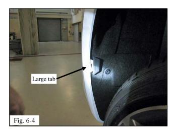
(d) Align the large tab on the bumper fascia with the receptacle inside the wheel well (Fig. 6-4).
